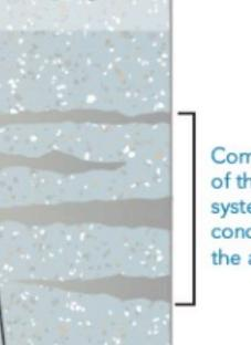
Compaction of the aquifer system is concentrated in the aquitards
