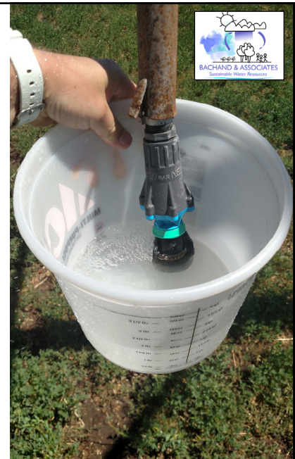
Measured time to fill 1 gallon, 4 tests per nozzle at 3 places in each span
